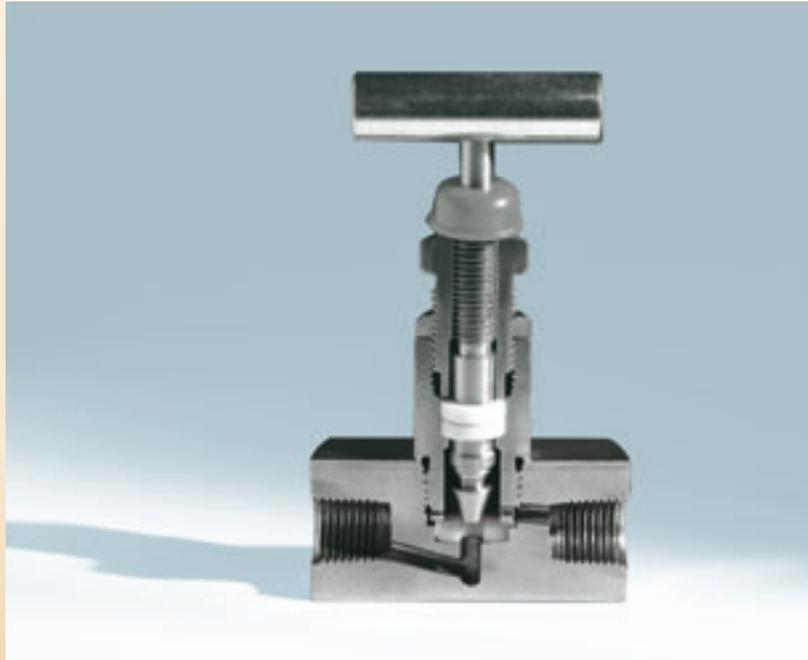
For applications where bubble-tight shutoff of liquids or gases are required. Pressure rating to 6,000 psi (42,000 kPa). These valves are designed with a replaceable Delrin\*\* soft seat.
