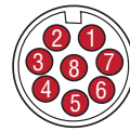
Integral D84 connector (male) as viewed from the end of the sensor
