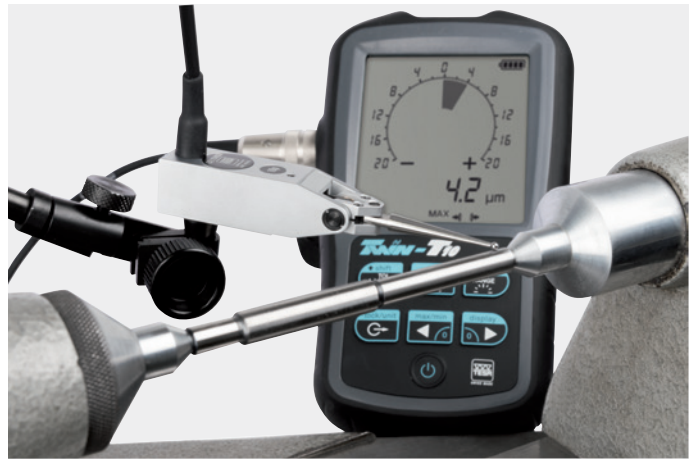
Run-out measurement with GT-31 lever probe
