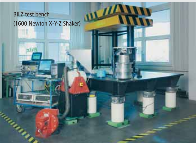
BILZ Democenter: Active Isolation System AIS™ with six degrees of freedom
