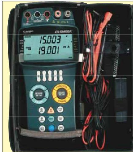
Carrying case lead cables for source/ measurement, terminal adaptor, 6 spare "AA" batteries, fuse, AC adaptor and instruction manual.
