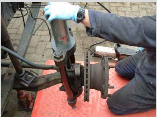
Replacing a sized king pin can be a time consuming process. Using the KPP20 means keeping trouble and labour time for this kind of job to a minimum.
