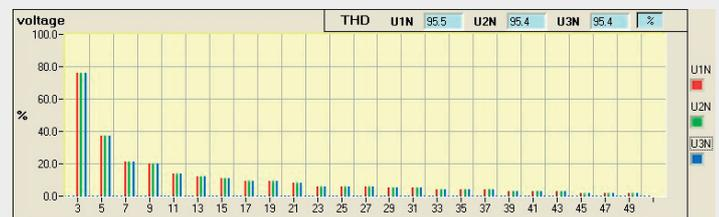
*Hint: The accuracy of the harmonic analysis depends strongly on the quality of the current and voltage transformers possibly used, because harmonics are normally heavily distorted. It's valid: The higher the frequency of the harmonic, the higher its damping.*
