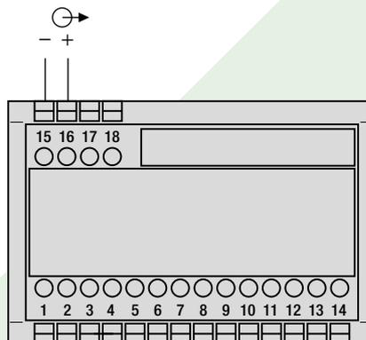
Fig. 6. Power supply internal from measuring input, without separated power supply.
