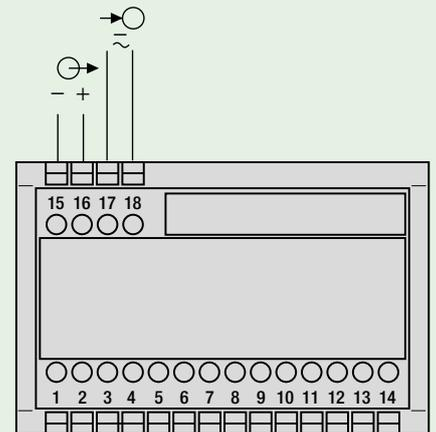
Fig. 7. Power supply connected to the low tension terminal side 17 and 18.
