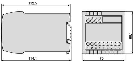
Fig. 8. SINEAX P530/Q531 in housing **P13/70** clipped onto a top-hat rail (35 x 15 mm or 35 x 7.5 mm, acc. to EN 50 022).
