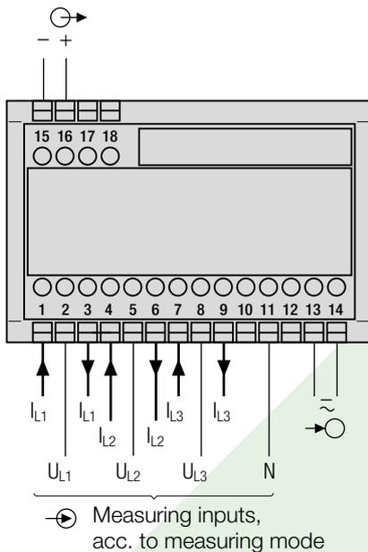
Fig. 5. Power supply connected to terminals 13 and 14.
