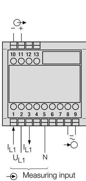
Fig. 2. Power supply connected to terminals 8 and 9.
