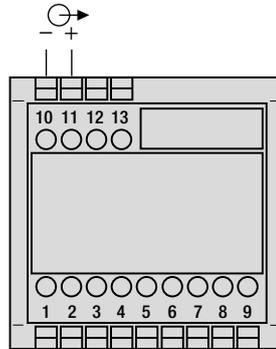
Fig. 3. Power supply internal from measuring input, without separated power supply.
