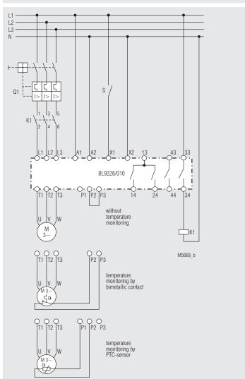
Auxiliary voltage U<sub>H</sub> = AC 400 V or AC 230 V
