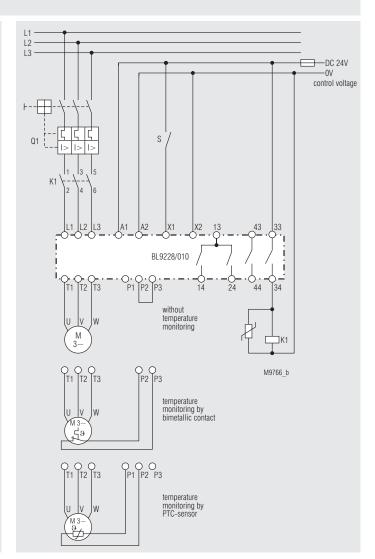
Auxiliary voltage U<sub>H</sub> = DC 24 V
