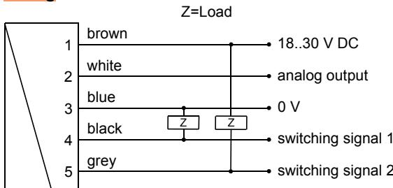
Before the electrical installation, it must be ensured that the supply voltage corresponds to the data sheet.
