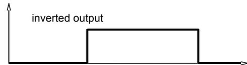
A Power-On delay function (ordered as a separate option) makes it possible to maintain the switching output in the normal state for a defined period after application of the supply voltage.
