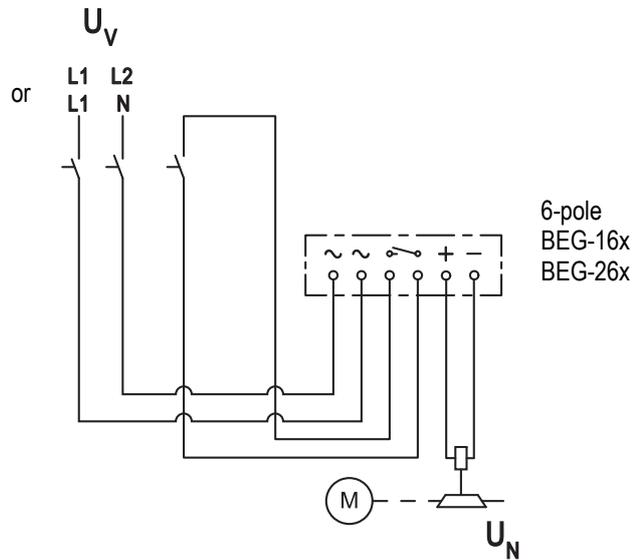
**Fig. 34:** Supply: Phase-phase or phase-N via 6-pole rectifier
