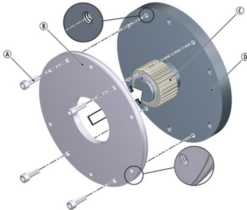
**Fig. 22: Flange mounting for sizes 18 – 20**
