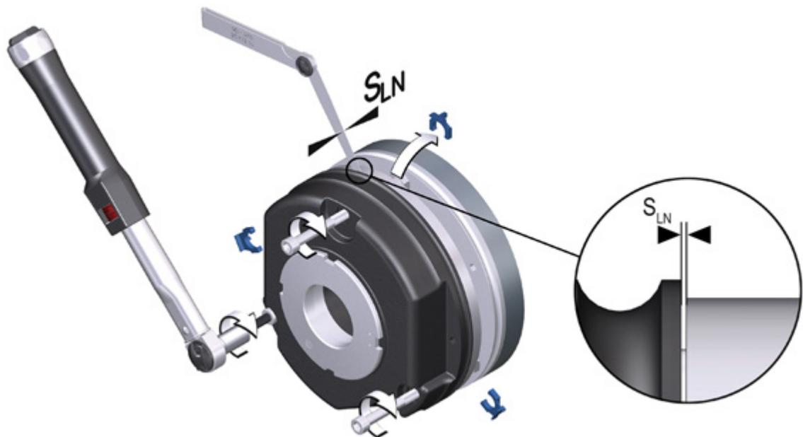
**Fig. 18: Tightening the screws with a torque wrench**
