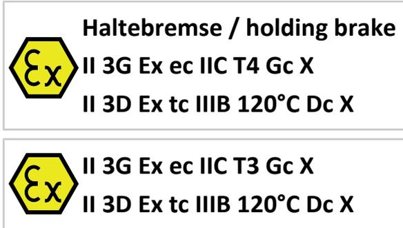
Fig. 14: Name plate ATEX holding brake (an example)
