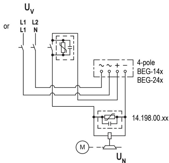
**Fig. 35:** Supply: Phase-phase or phase-N via 4-pole rectifier
