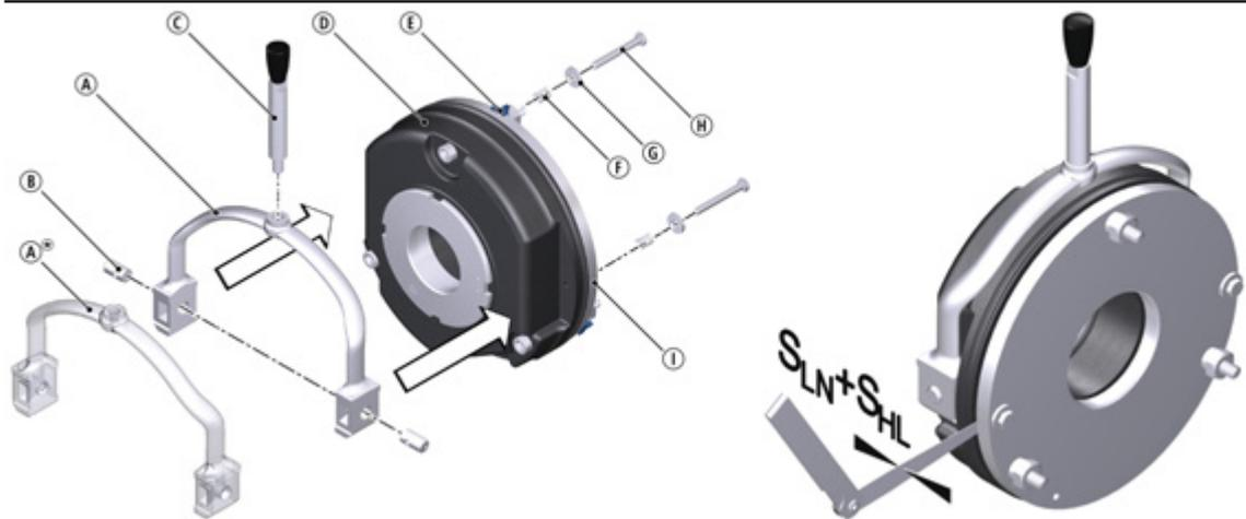
Fig. 27: Assembly of the hand-release BFK458
