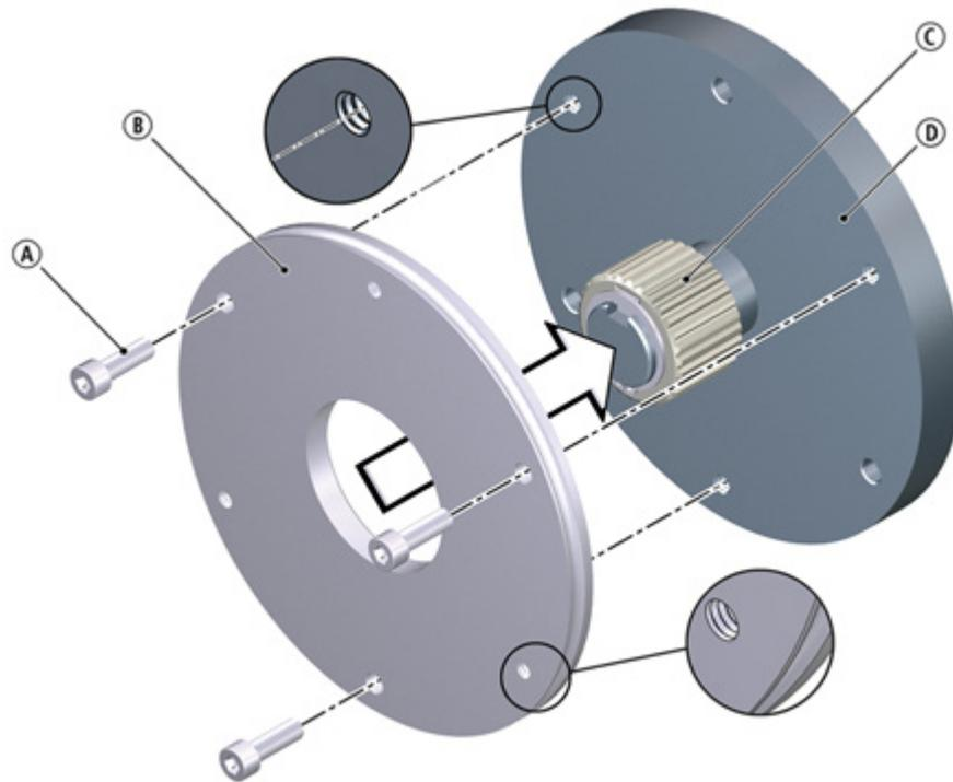
**Fig. 21: Flange mounting for sizes 06 - 16**
