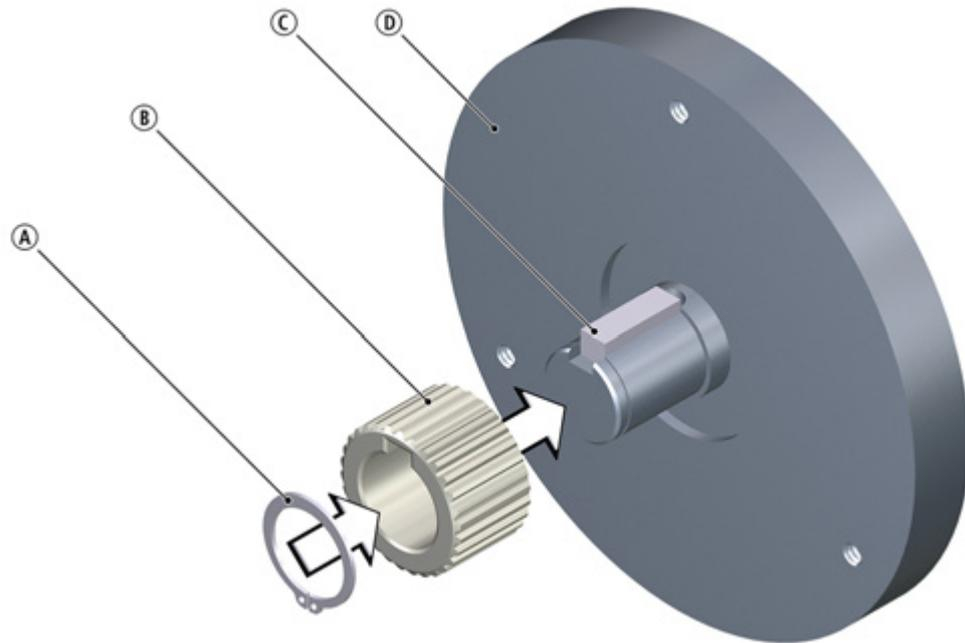
**Fig. 15:** Installing the hub onto the shaft
