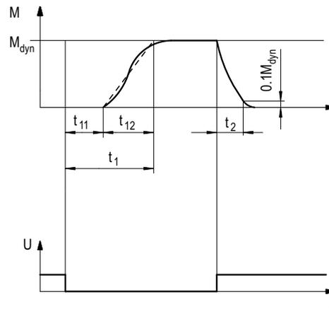
**Fig. 4:** Operating/switching times of the spring-applied brakes
