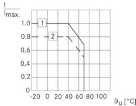
**Fig. 37: Permissible current load**
