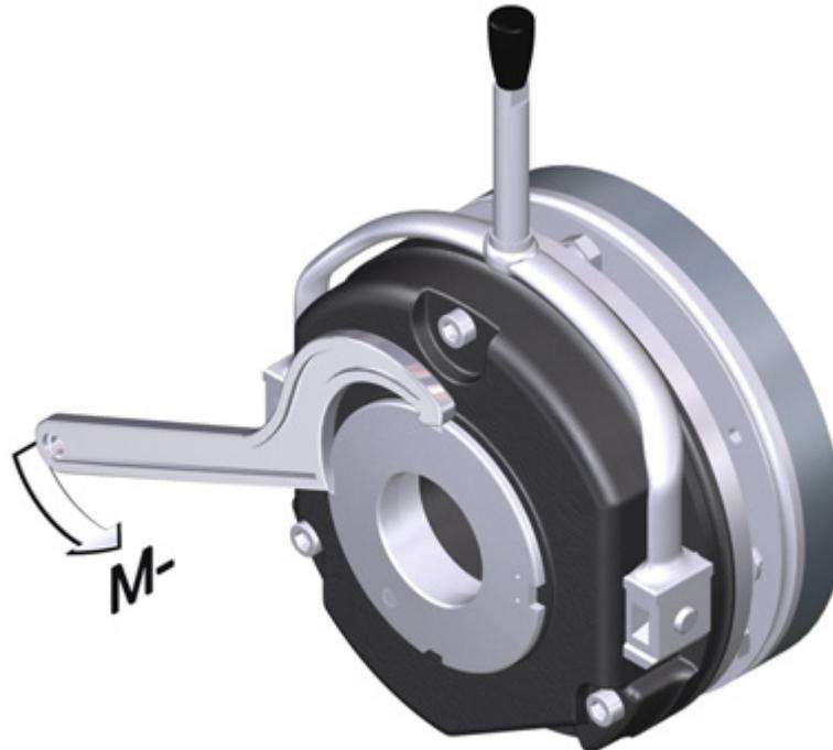
Fig. 39: Reducing the braking torque
